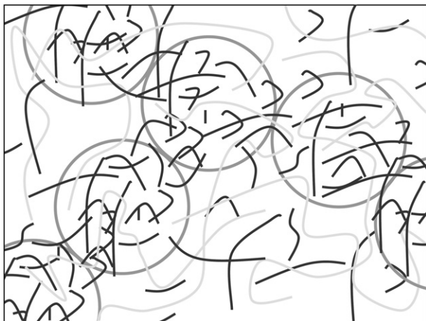
Fig. 12. Schematic of the microstructure of polycarbonate/carbon nanotube composites: agglomerates of entangled nanotubes (indicated by circles) that cluster and constitute electrical conductive pathways are embedded in the polymer matrix.
